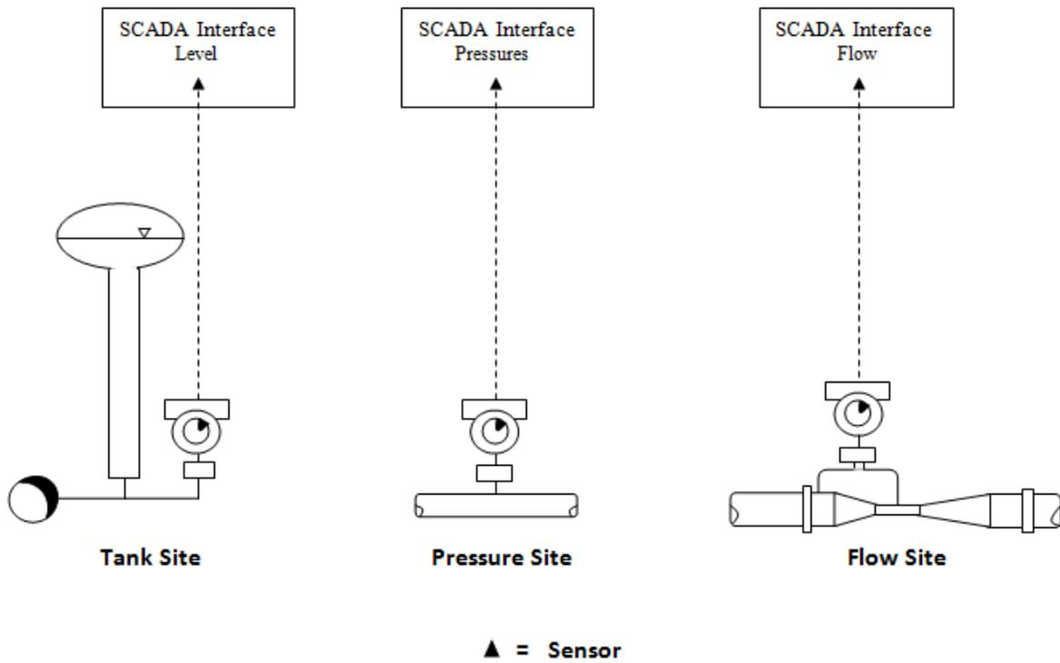
**Typical instrumentation for level, pressures and flow monitoring sensors**
